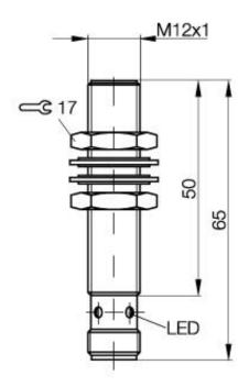
Inductive Sensors BES M12MI-PSC40B-S04G M12x1 x 65 normally-open Sn=4mm shielded
